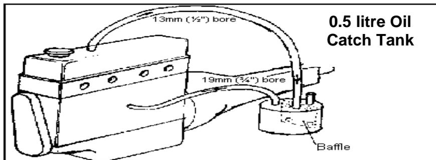
An oil catch tank, with a minimum capacity of 0.5 litres, must be fitted in the engine bay, and must have a minimum of two breather pipes connecting to it, one from the rocker box and one from the crank case. If the catch tank becomes ineffective during racing or practice, the car will be withdrawn from the event.
