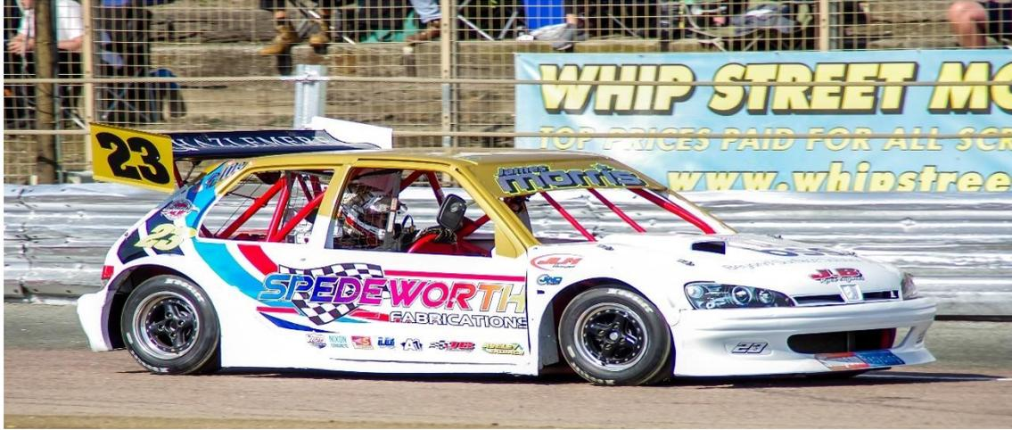
**A.** Any four-seater, front-engined, saloon or hatchback, constructed of steel, the overall length must not exceed 3988mm (157") and the overall width must not exceed 1702mm (67") when ready to race. Consideration will be given to any modern vehicle which falls outside these specified measurements in its original form, but can comply when prepared for racing, as follows:
